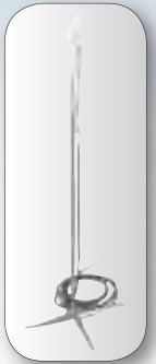
Detail of the methane combustion torch.
